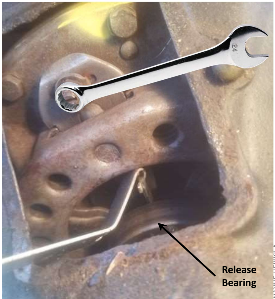
Figure 3: Adjust six clutch fingers to 5/8"
