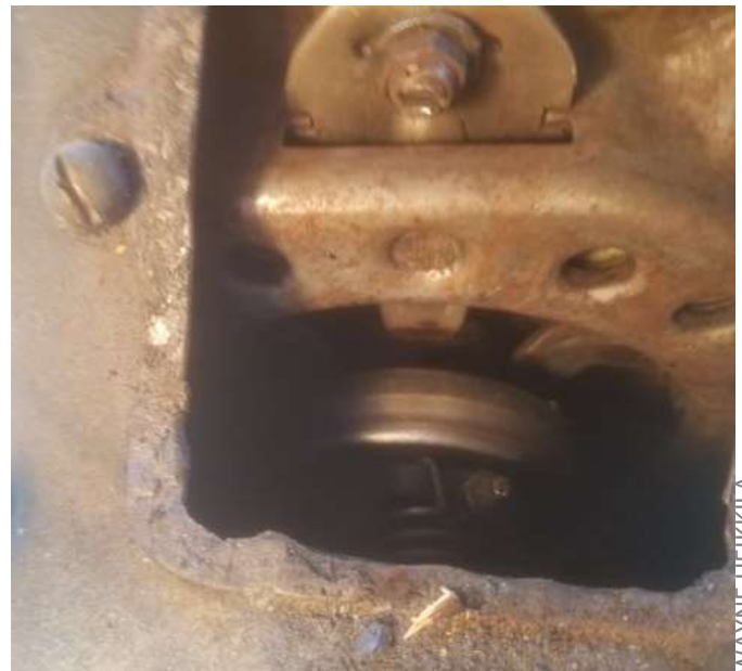
Figure 1: Floor Removed and Clutch housing hand hole cover opened
