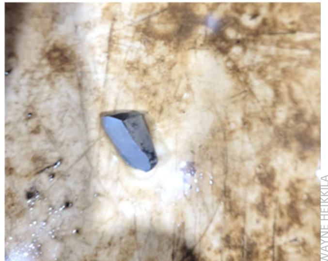
Pieces of gear metal falling out in a transmission fluid change is not a good sign
